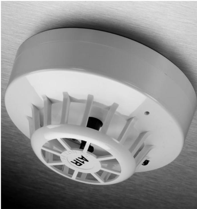
increases rapidly the resistance of the exposed thermistor becomes less than that of the insulated thermistor. The ratio of the resistance of the thermistors is monitored electronically and an alarm is initiated if the ratio exceeds a factory preset level. This feature determines the 'rate of rise' response of the detector.
